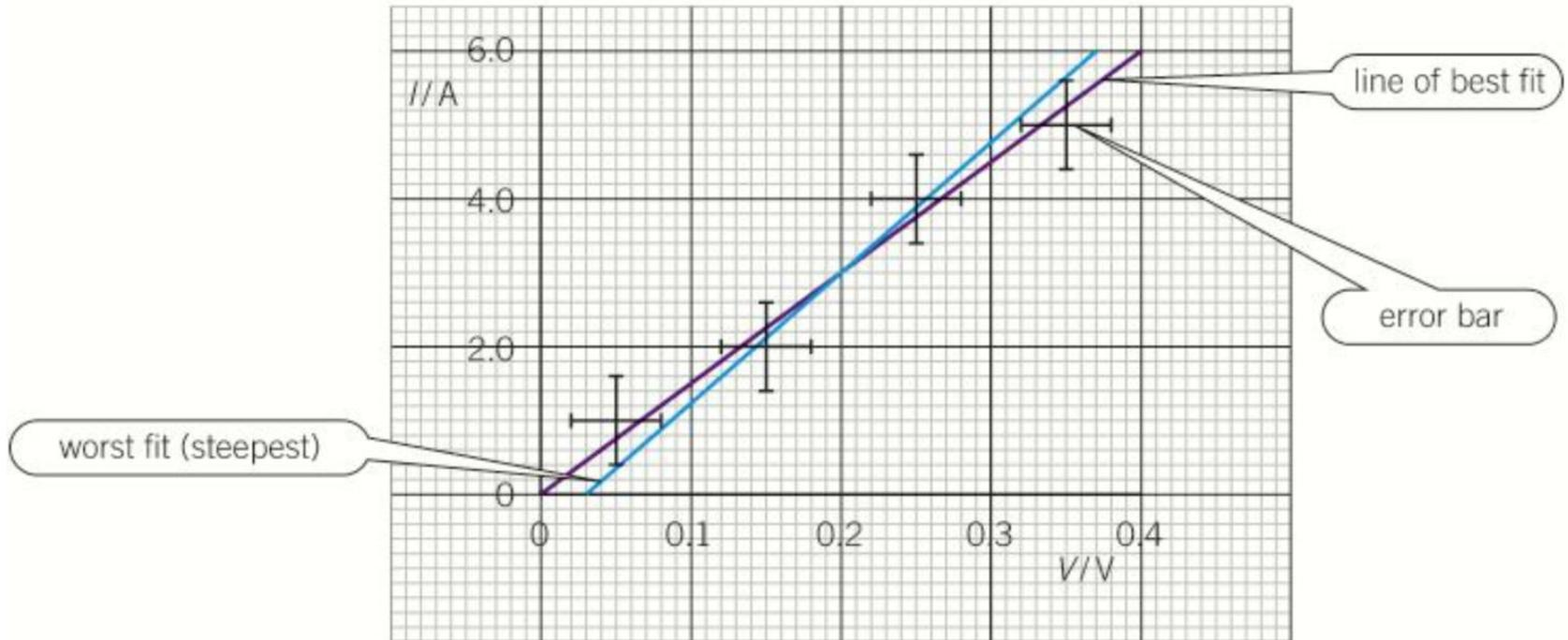
The absolute uncertainty in the gradient is the positive difference between the gradient of the line of best fit and the gradient of the line of worst fit.
